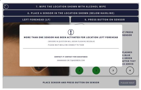
The Multiple Sensors Activated Alert Warning will appear if you activate more than one Sensor while placing Sensors on the scalp during the Sensor Placement procedure. The REMI Tablet will automatically turn off the conflicting activated Sensors and ask you to repeat the current placement. The SNOOZE button will appear when the REMI Tablet has reset the Sensors.
