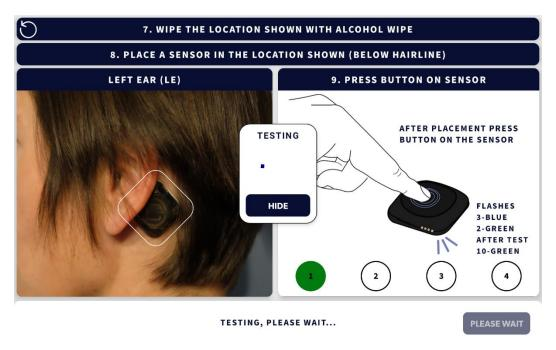
The REMI Tablet will instruct the REMI Sensor to test the electrode contact quality (ECQ) between the Sensor and the scalp. If the ECQ is good, the Sensor will flash its LED green 10 times; REMI-Mobile will automatically reset the TEST button to PLEASE WAIT and change the left image to the next Placement location. If the ECQ is bad, an alert will appear. Please see the Poor Electrode Contact Alert section. Repeat the Placement and Testing
