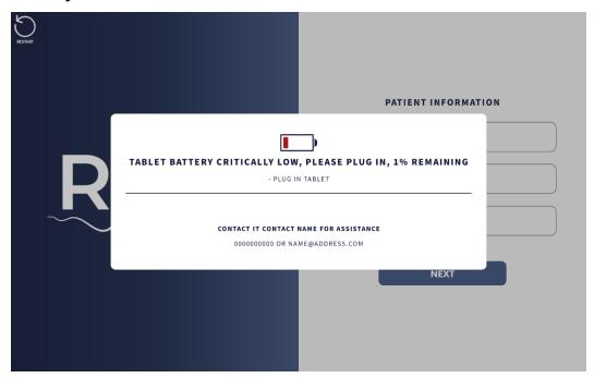
It is recommended that the REMI Tablet be plugged into A/C power at all times. Should the battery reach 50% capacity or less and is not plugged into A/C power, an alert screen will appear. All REMI Sensors will begin to flash their LEDs alternating red and blue. If REMI Tablet battery power is above 25% you will be able to "snooze" the alert screen.
